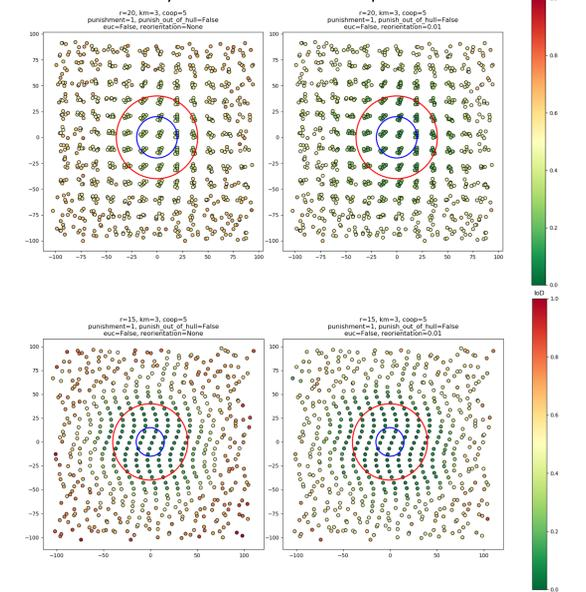
Results from applying two versions of the IoD algorithm without and with realignment (left and right respectively) to synthetic patterns. The pattern is perturbed with random noise that increases in strength as a function of distance beyond the red circle, and the blue circle represents the neighborhood size. Realignment enables better detection of discrete patterns, such as the top pattern, but often reduces differentiation for continuous patterns, such as the pattern on the bottom.
